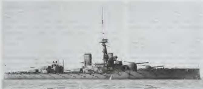
Figure 30: HMS Orion, super dreadnought battleship of the Royal Navy. Heavier than HMS Dreadnought but just as fast, this ship mounted 10 13.5-inch guns of greater armour-piercing power in five turrets along the centreline of the vessel. The Orion was present at the Battle of Jutland in 1916 and was scrapped under the Washington Treaty of 1922.
